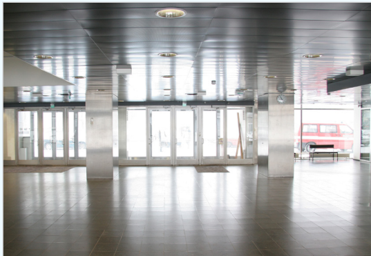
Fig. 16. Strong lights are coming through windows and reflecting off a reflective floor, causing glare and reduced visibility.
