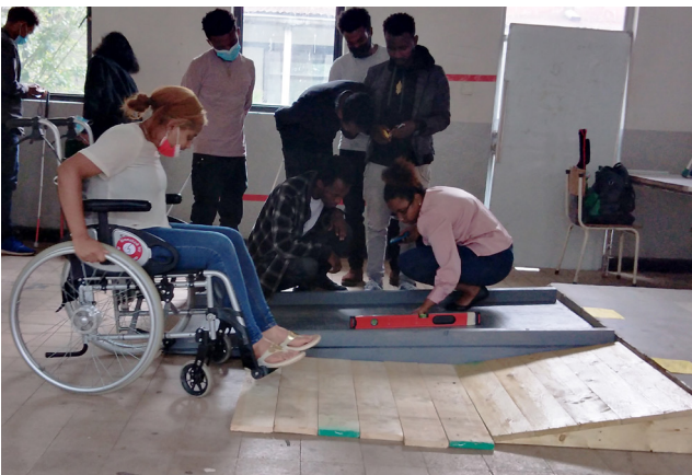
Fig. 2. A student is using a wheelchair and testing different surfaces and slopes of a ramp to assess how easy or difficult it is to move in the built environment.
