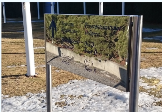
Fig. 26. Example of a sign with a shiny and reflective surface, which makes it difficult to read the text.
