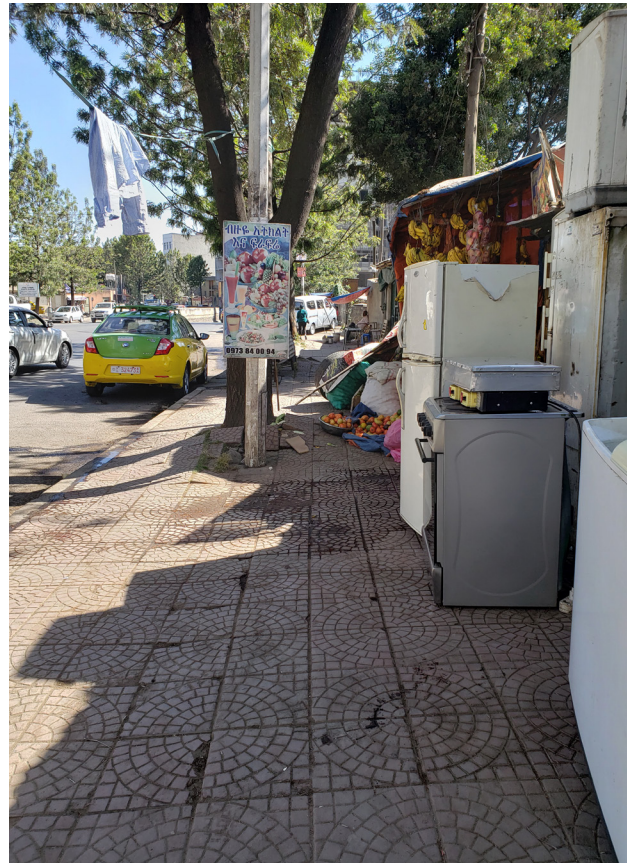
Fig. 30. Misuse of space. This pathway is difficult to navigate due to vendor stalls, obstacles and trees located on the walking route. There is also a lack of visual and tactile cues on the pathway.
